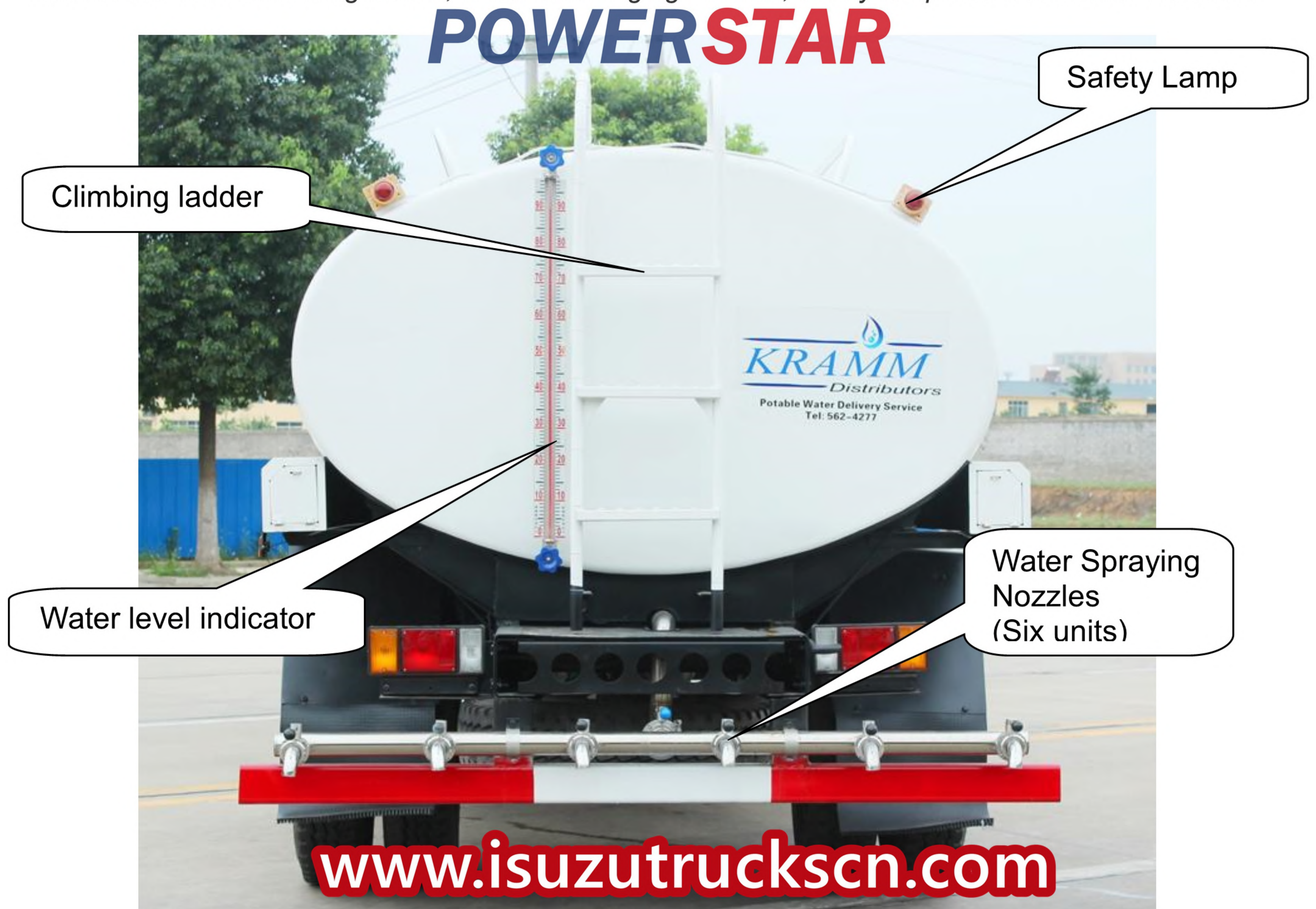
Rear of the Tank: Climbing ladder, water discharging nozzles, safety lamp and water level indicator.
